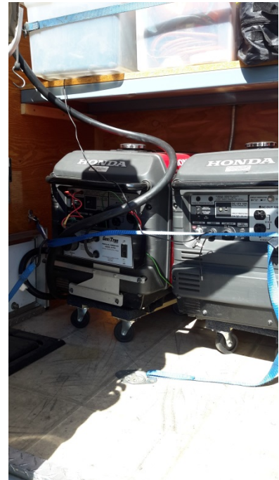
Portable Generators to power Search & Rescue Command Post Trailer Generator 134 lbs. each; 2 person lift
