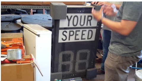
Speed Sign 54 lbs. Lifted manually into bucket truck.
