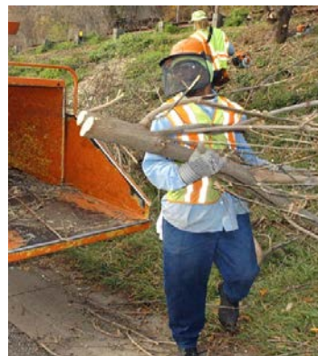
Limbs up to 6 inches diameter into chipper. Approximate weights from 50 to 75 lbs.
