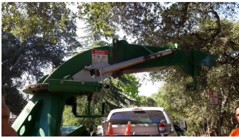
Exit shoot for chips. 46 lbs. push force to move.
