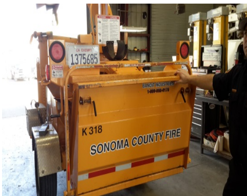
Wood Chipper Feed Chute- Closed Lift force- 63 lbs. to lift and close
