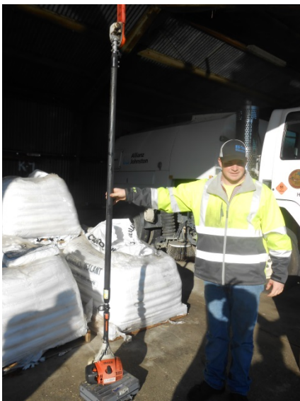
Pole Saw – 17 lbs. Shortest at 107” Extends to max of 180” (15’)
