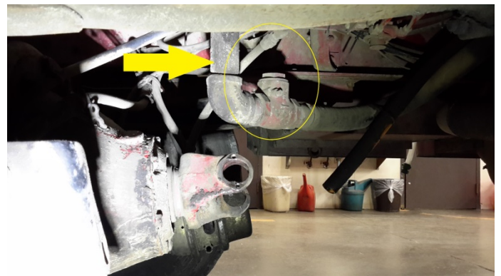
Under carriage of Fire Truck- Water Pump Mount Circled
