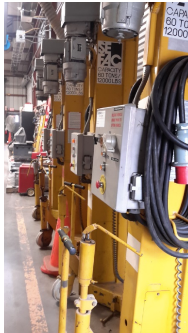
SEFAC- Mobile Column Lifts Pull Force – 66.5 lbs.
