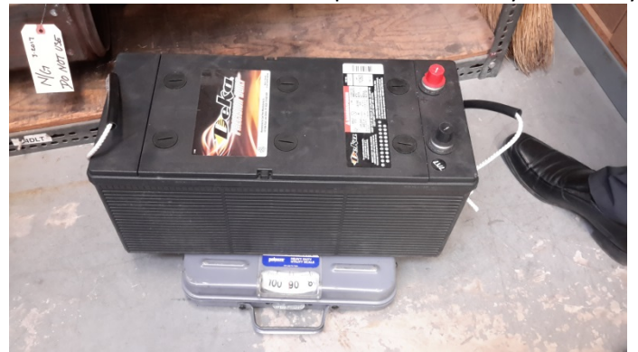
Truck/Heavy Equipment Battery - 93 lbs. Stored on 3 inch shelf (can be difficult to manage in field)
