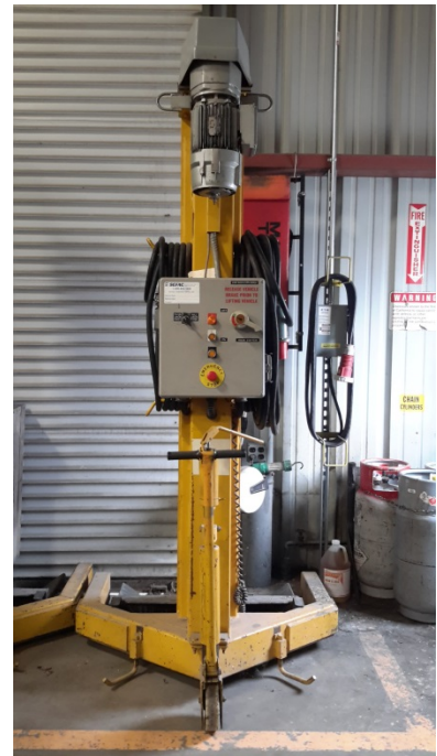
SEFAC- Mobile Column Lift Push Force – 61.5 lbs.
