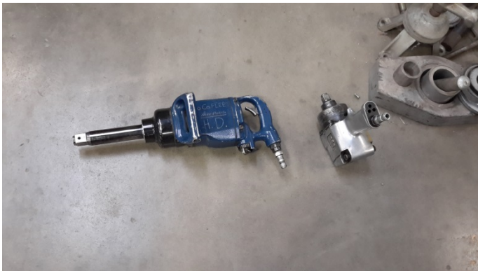
1" Drive Truck Tire Impact Wrench (blue)-27 lbs., as shown 3/4" Drive Truck Tire Impact Wrench (silver)-12 lbs., as shown
