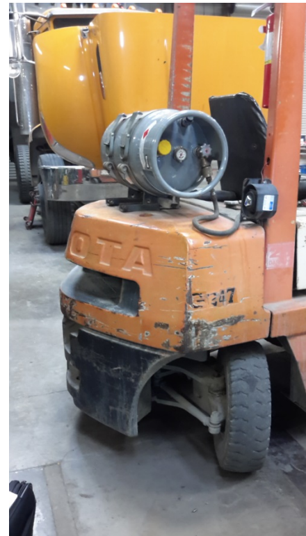
Propane powered Forklift Tanks lifted to 45" high to change
