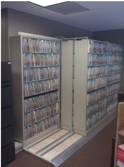
Example of sliding file storage Top shelf at 69 ½ inches high Push/Pull force- 17 lbs.
