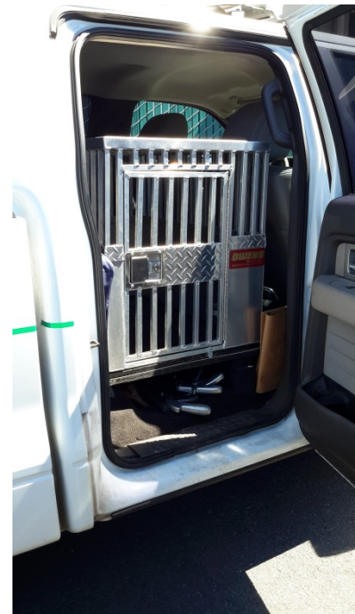
Animal Cage in back of Duty Vehicle -floor of cage at 32 inches
