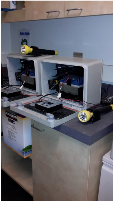
Radar Recorder Kit- 40 lbs. Stored on 39 inch counter top Carried 25' to Duty Vehicle Installed at 72 inches or above ground
