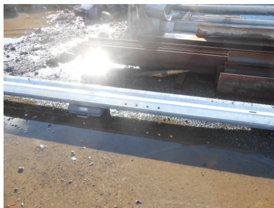
Guard Rails- typical = 91 lbs.
