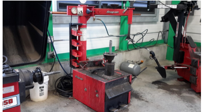
Tire Mounting Machine- 42 inch lift to clear shaft with rim and tire
