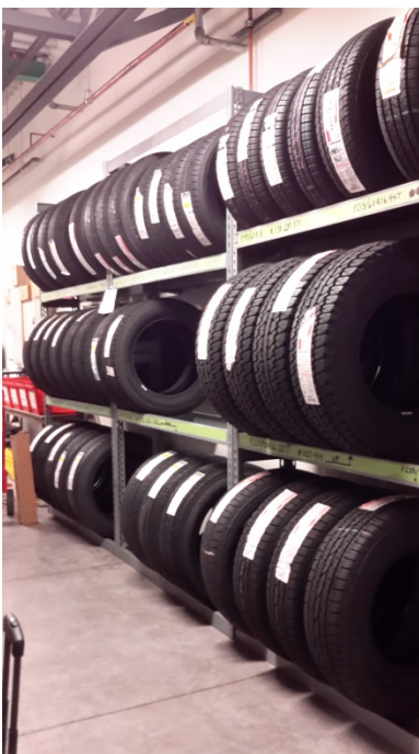
New Tire Storage- Various Sizes Most commonly used tire-18lbs. Tires stored up to 72 inches high
