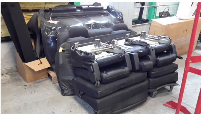
Stack of Back Seats removed from Patrol Vehicle to install Molded seats (stored and re-installed prior to auction)
