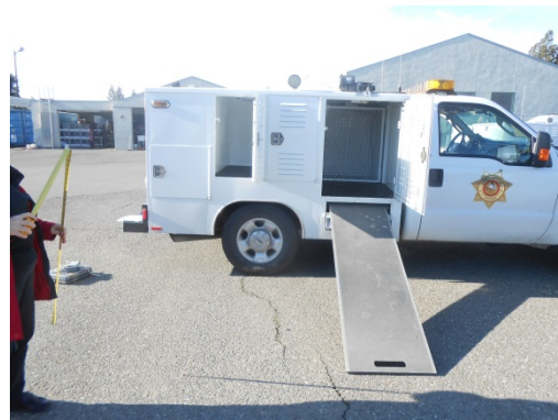
Cage Compartment - Small, 41 inches high Large/Ramp- 34 inches high
