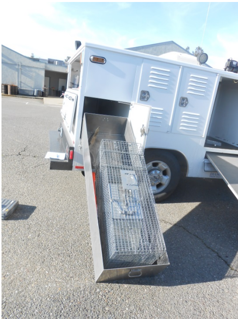
Dead Box with Trap- 51.5 lbs. pull force, Assuming 30 lbs. animal
