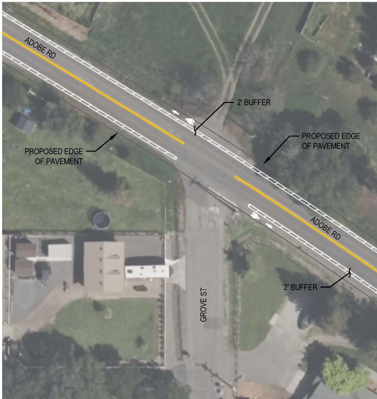
Figure 2.6 Phase 2 Proposed Lane Narrowing & Buffered Bicycle Lanes on Adobe Road (East of Main Street)
